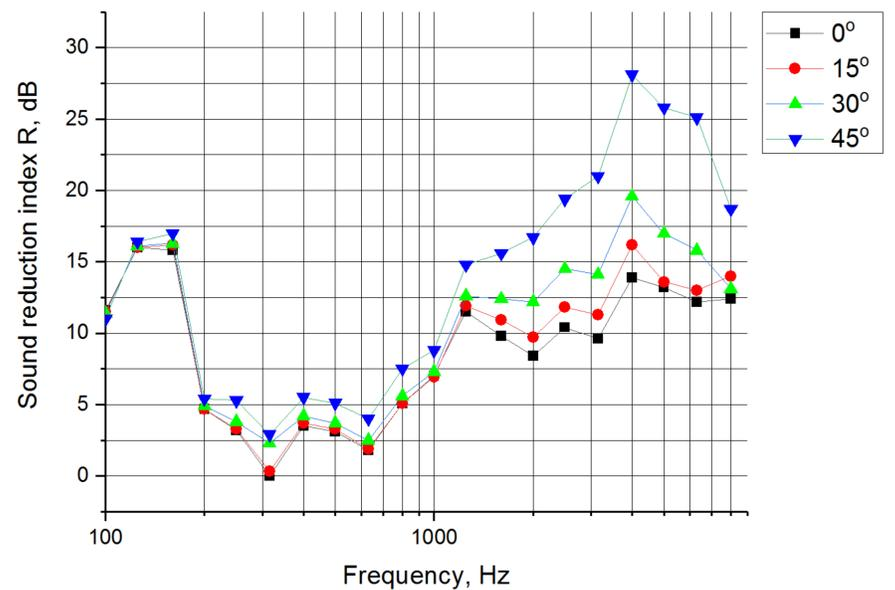
Fig. 5. Sound reduction index using 1/3 octave band filter of acoustic louver covered with 20 mm foil-faced pressed rockwool
