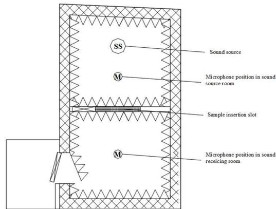
Fig. 1. The design of semi anechoic chamber
