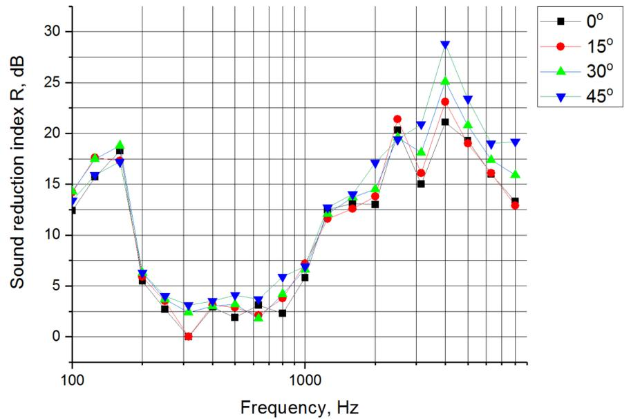
Fig. 4. Sound reduction index using 1/3 octave band filter of acoustic louver covered with 30 mm pressed rockwool
