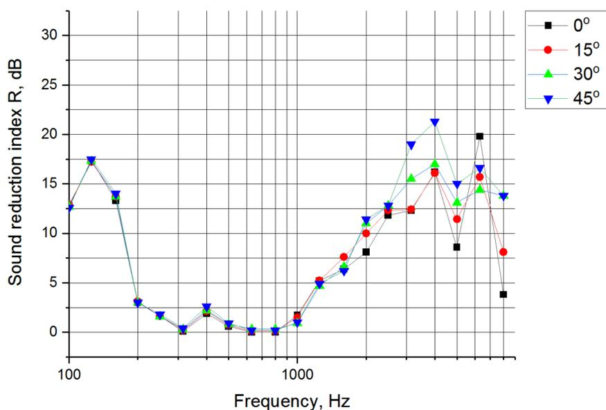
Fig. 3. Sound reduction index using 1/3 octave band filter of acoustic louver covered with 20 mm pressed rockwool
