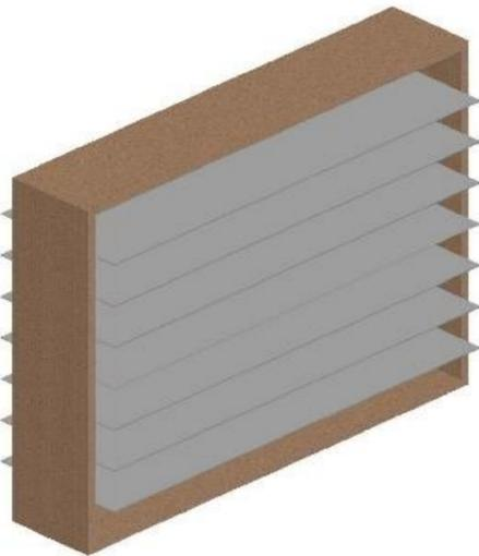
Fig. 2. The design of acoustic louver frame
